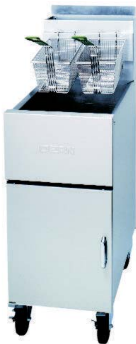
SM50G gas fryer standard with 120,000 BTU (30,600 kcal) (35.2 kW) burners and 35-50 lbs. (20-28 L) oil capacity (shown with optional casters).
