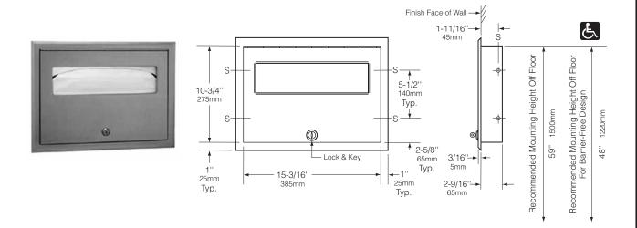
Rough Wall Opening 15-5/8" (395mm) wide 11-1/4" (285mm) high 2-5/8" (67mm) minimum recessed depth
