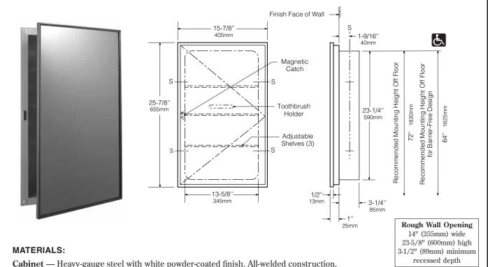
Door — Heavy-gauge steel with stainless steel channel frame. Secured to cabinet with an enameled steel pia
