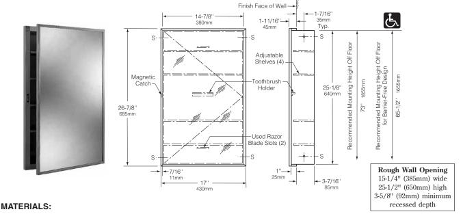
Cabinet — 18-8 S, type-304, 22-gauge (0.8mm) stainless steel. All-welded construction. Two slots for used razor blades.
