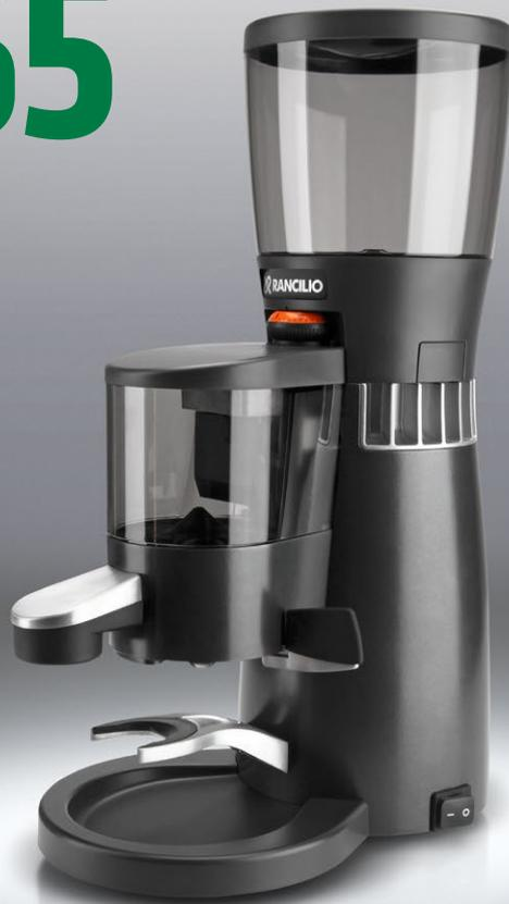
**KRY065** is fitted with 2.5 inch (64mm) diameter burrs, ensuring a production of 15-20 lb/h (7-9 kg/h). The dose can be regulated between 0.19 and 0.35 oz (5.5-10 g), with a coffee bean capacity of 2.9 lb (1.3 kg). It is available in an automatic (AT) or semiautomatic (ST) version.
