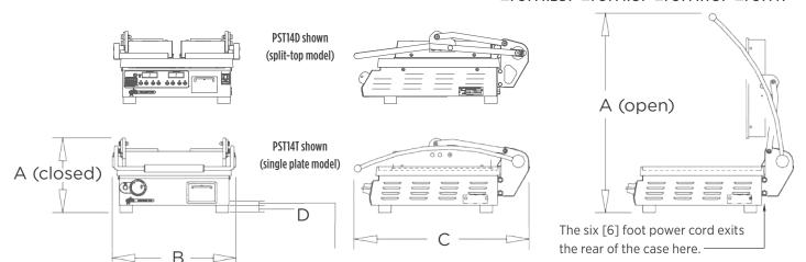
The cord exits approximately .625 in. (159 mm) up from the base of each model and from the right side [looking from the front] the cord is 1.5 in. (38 mm) from the side on the 7-in. model and 3.375 in. (86 mm) on the 14-in. model.
