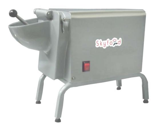
Compact unit designed for shredding and grating cheese and vegetables. The RQ-150 makes short work of all types of cheese both soft and hard. 3/4 HP motor drives a 6" blade at 485 rpm. Motor housing stainless steel, enamel finish aluminum hinged feed door. Unit comes standard with four blades, three shredding 1/8", 3/16" and 5/16" and one hard grating blade. It also comes with a catch pan that easily fits under unit.
