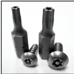
Exterior Fasteners are Tamper Proof Torx Pin Screws
