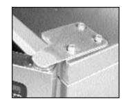
**HEAVY-DUTY 1" STAINLESS** STEEL TUBULAR HINGE .... Full length eliminates torque on top hinge. Mounted with 1" bushing and 12 gauge stainless steel mounting bracket. Keeps doors properly aligned and withstands rugged use.
