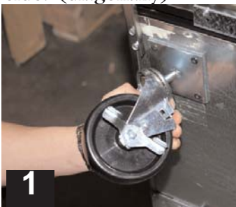
1 Thread castor into the underside of cabinet frame rail.
