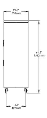
Minimum Wall Clearance Both Sides and Back -6 inches (152 mm)
